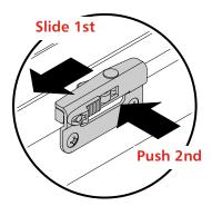
1 To fully open sash, disengage window opening control device.
