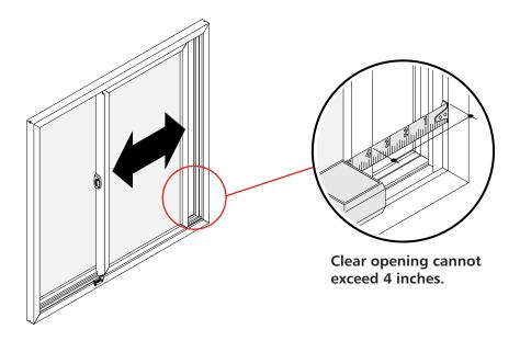
Window opening control device application procedure is completed.
