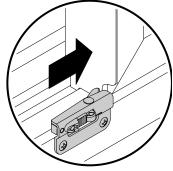
3 Close sash. Window opening control device automatically resets.
